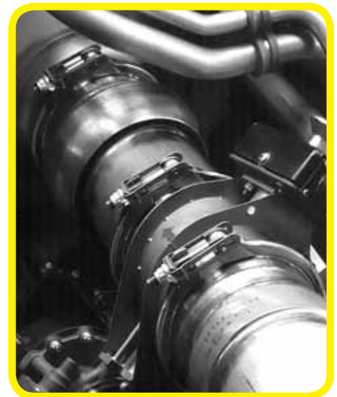
Fig. 6 — Typical high-pressure pneumatic ducting connection
