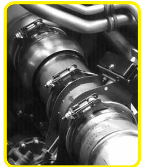
Fig. 6 — Typical high-pressure pneumatic ducting connection
