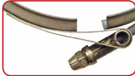
*Fig. 14b — Tangential Backbend*
